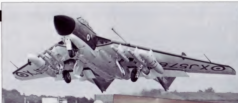
Above: An FAW.Mk 1 leaps into the air from a land base, carrying four dummy Firestreak missiles and the outer pylon fuel tanks that were a standard feature.
